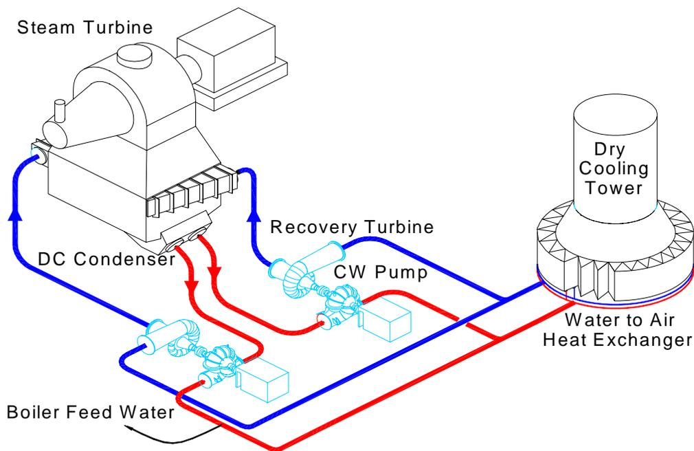
**Schematic diagram of indirect dry condenser cooling system.**
