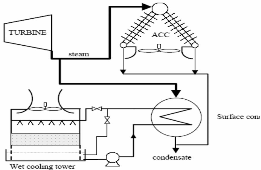
**Schematic diagram of hybrid cooling system with ACC.**
